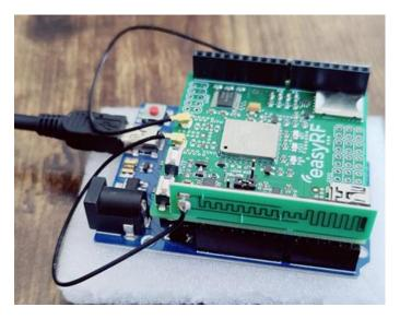
Verify the Arduino board is recognized by the PC/Laptop, and upload an example of your choosing to the Arduino board. When opening the COM port in the Arduino software, make sure to put it on 9600 baud.
